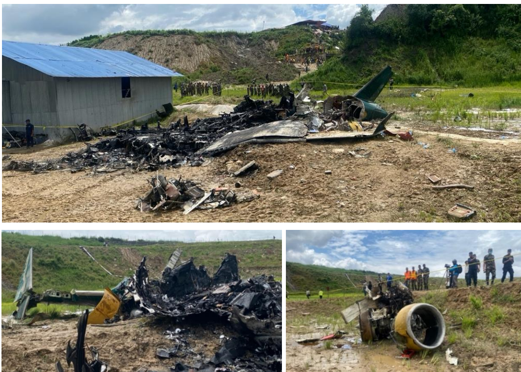
Figure 2: Top: scene at '5', with '4' just above on the hill, bottom: burnt fuselage and empennage sections at '5' and left engine at '2'
