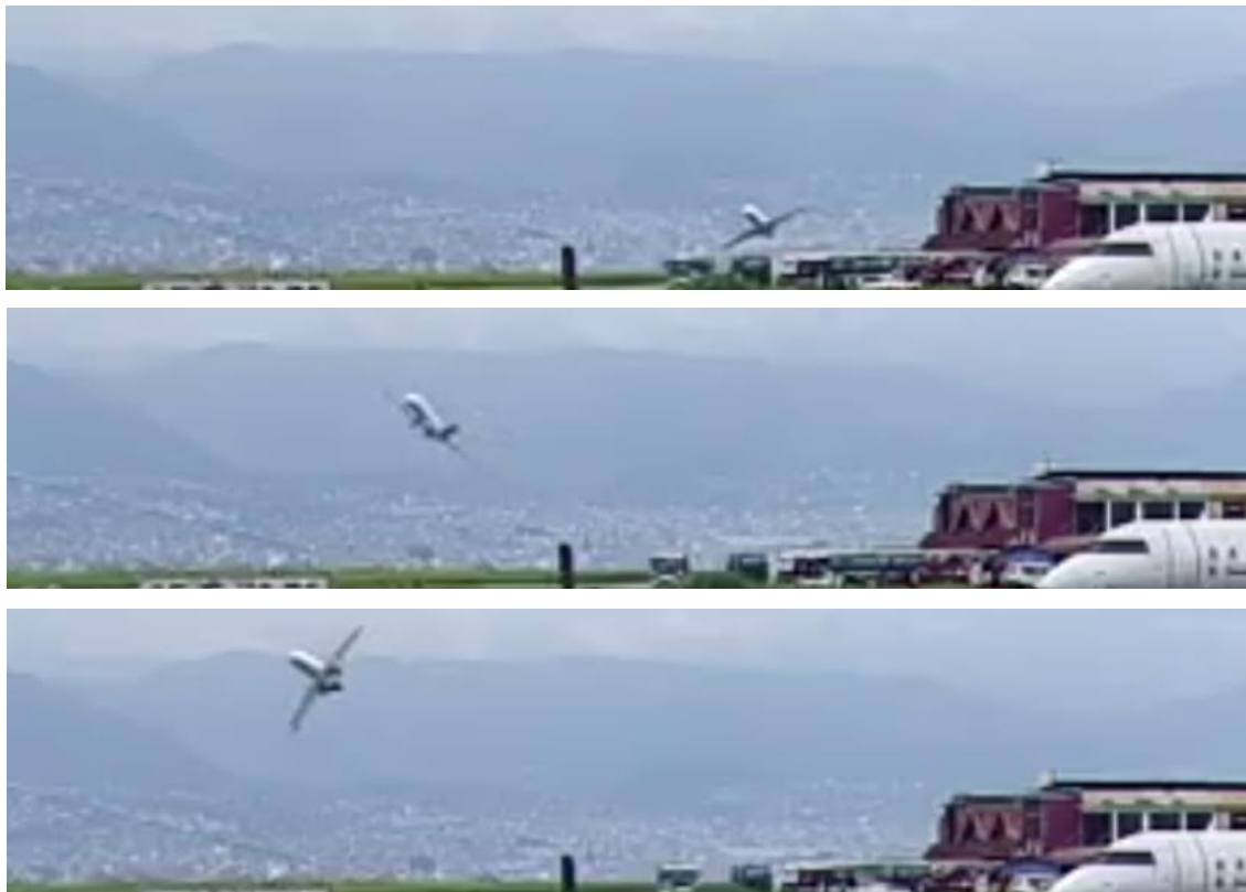
Figure 7: Event sequence with unusual attitudes leading to the accident, captured by a CCTV camera. Almost immediately after rotation, the aircraft first went into a right wing down attitude, followed by left wing down-right wing down sequence. This sequence can be discerned from Figure 7. In
